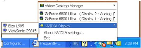
**3** Click **NVIDIA Display** (Figure 4.5) and then select the type of display. The NVIDIA Display control panel appears (Figure 4.7).
