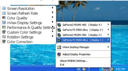
Figure 4.6 NVIDIA Settings Sample Menus with Four Connected Graphics Cards
