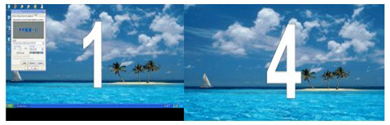
**Note:** You can repeat steps 4 and 5 and chose Vertical Span or Clone mode. The result will be similar to what is shown in Figure A.7 and Figure A.8 in that the secondary displays become detached because nView Span and Clone modes do not detect the secondary display as a separate display.
