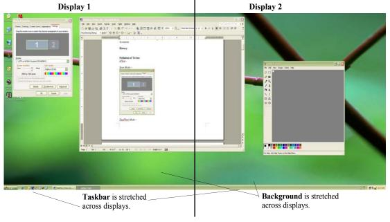
Figure 5.9 Multiple Displays in nView Horizontal Span Mode
