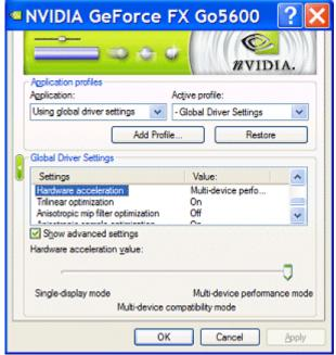
• Multi-display compatibility mode is available if you have two or more active displays when running in nView Dualview display mode or if you are using different classes of NVIDIA GPU-based cards.
