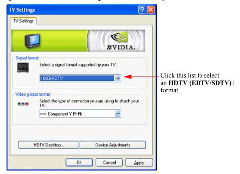
Figure 7.2 HDTV Overscan Configuration — HDTV Component Connection
