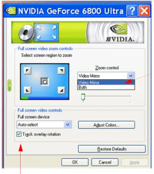
**Zoom controls** apply to the display being used for the "video mirror" feature.
