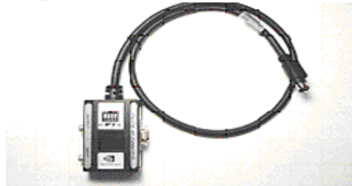
10-pin to VIVO Pod with D-Connector
