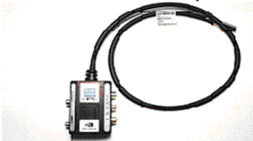
10-pin to VIVO Pod with Component
