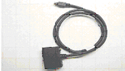
10-pin to VIVO Pod with Component
