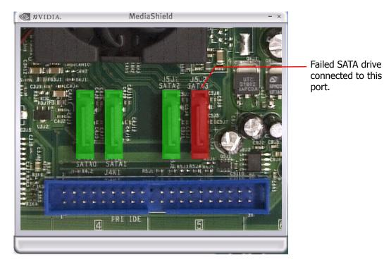
Figure 5.3 Disk Alert Example—Failed SATA Drive
