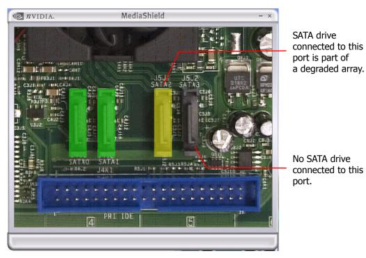
Figure 5.2 Disk Alert Example—Degraded and Missing SATA Connection
