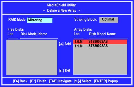
Figure 2.6 MediaShield Utility—Array Disks Assigned
