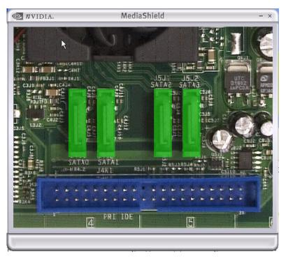
Figure 5.1 Disk Alert Example—All SATA Drive Connections OK
