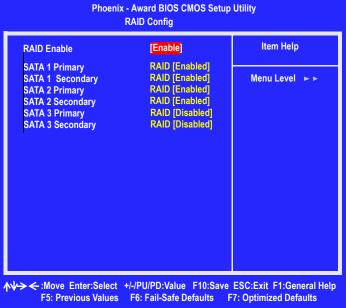
Figure 2.3 RAID Config Window
