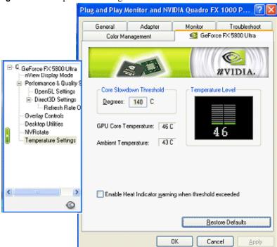
Figure 9.28 Temperature Settings Panel
