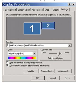
Figure 5.11 Windows 2000 Display Settings: Dualview Mode (Display 2 attached)
