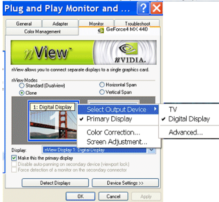
Figure 7.13 nView Clone Mode (Display 2 = Analog Display): Windows 2000
