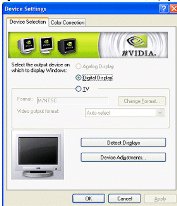
Figure 7.9 nView Device Selection Panel (Display 2 = Digital Display)
