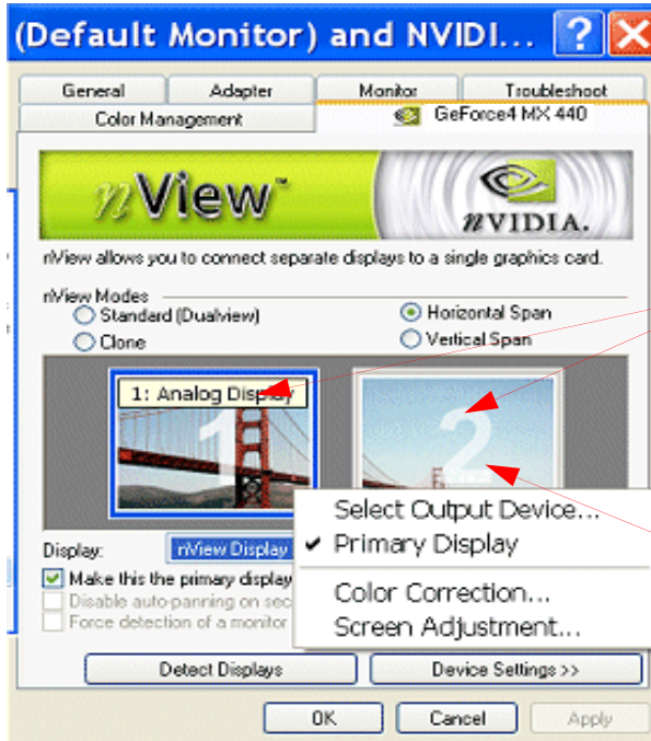
Figure 7.17 nView Horizontal Span (Display 2 = Digital Display) Windows XP
