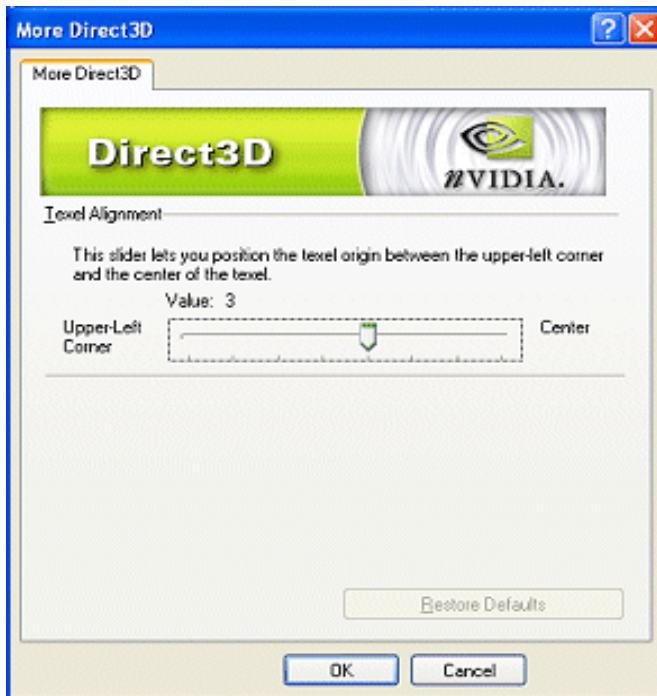
Figure 9.13 More Direct3D Settings: Texel Alignment (applies to older NVIDIA GPUs)
