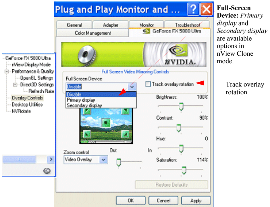
Figure 9.21 Overlay Controls Panel: nView Clone Mode
