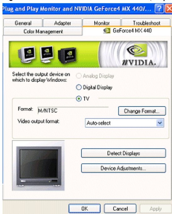
Figure 7.11 nView Device Selection Panel (Display 2 = TV)
