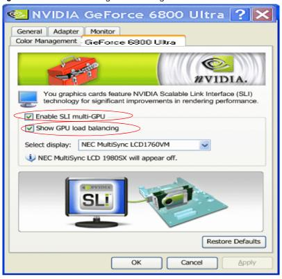
Figure 7.37 NVIDIA SLI Page — Enabling SLI Multi-GPU
